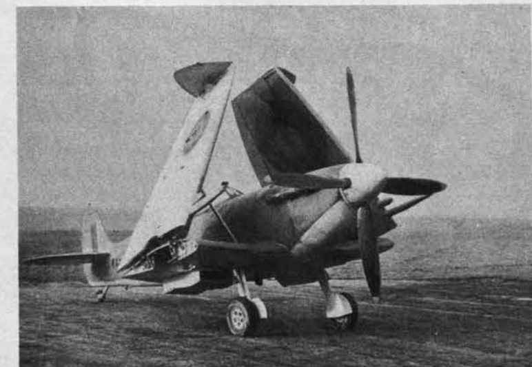
pointed rudder of the later Spits. The Seafire III (right) has a similar tail. Its new features include a four-bladed propeller, a special folding wing and the semi-blister canopy found on Spitfires XII, XIV and 21.
